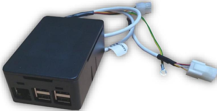
The **cMDB** (Cartadis **m**ulti-**d**rop **b**us) is the Cartadis MDB controller for **Gespage**. This companion is the physical link connecting a vending machine to a Gespage server.
